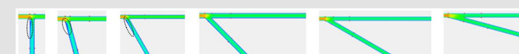
Figure 5: Separation zone for different offtake angles ( from left 90, 75, 60, 45, 30 and 15 degree)
