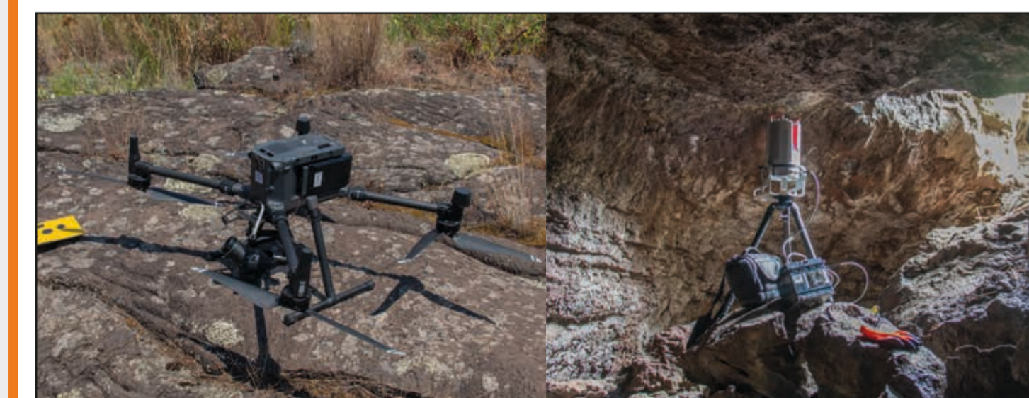
Figure 5. Scanning devices. a) UAV equipped with an optical camera; b) Riegl VZ-400 terrestrial laser scanner
