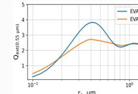
**Figure 4:** Mie extinction efficiency at 550nm for EVA1 and EVA2.
