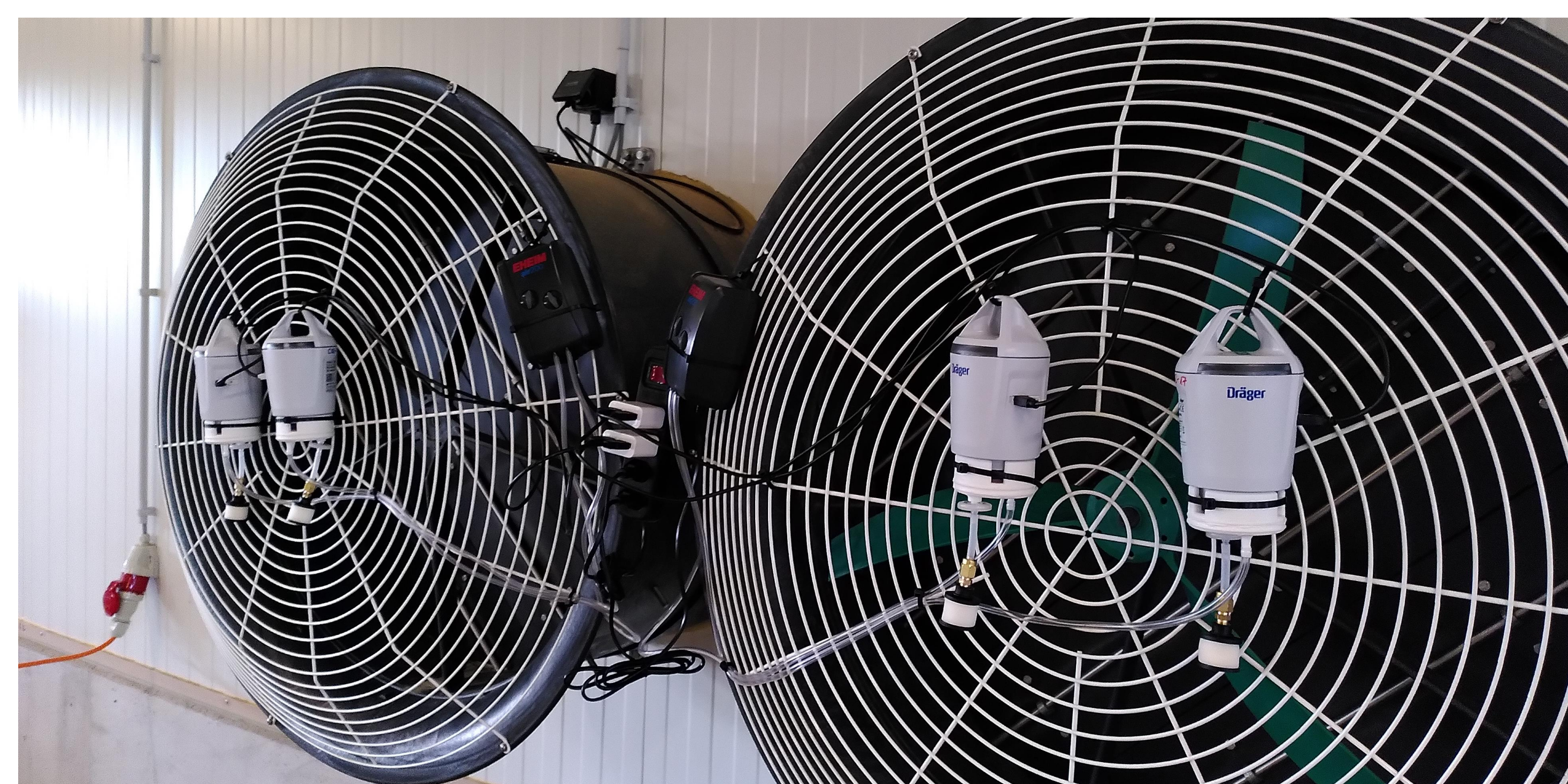
NH 3 / CO 2 sensors and measuring fans in front of two air outlet fans
