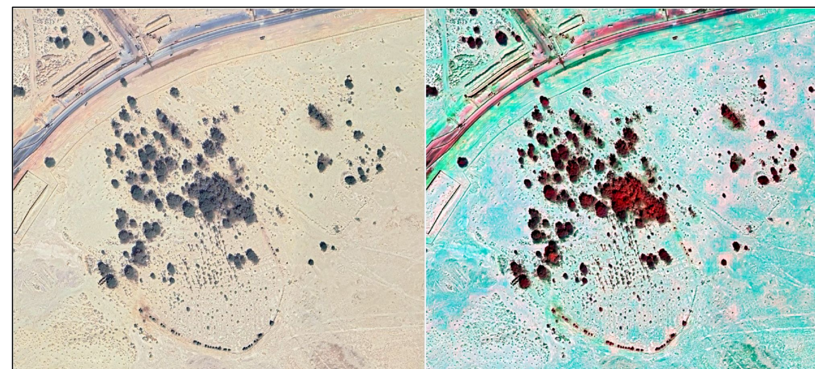
NIR composite (right) created from an RGB image (left) using an estimated NIR band using the deep learning model. The vegetation response resembles that of a composite produced by a satellite image with an actual NIR band.
