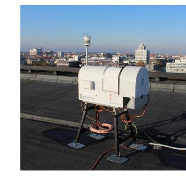
A microwave radiometer (HATPRO-G5, RPG Radiometer Physics GmbH) provides vertical profiles of air temperature and absolute humidity up to an altitude of 10 km. Integrated liquid water path (LWP) and the integrated water vapor (IWV) are derived from measurements of the brightness temperature in 14 channels.
