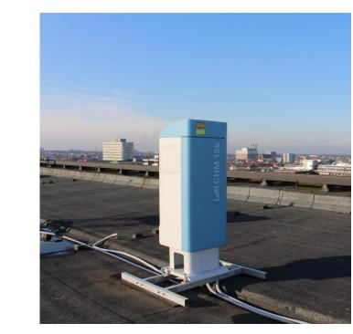
Cloud height, cloud cover and aerosol layers are recorded since 2017 with ceilometers (CHM 15k, Lufft) at sites Grunewald and TUCC, which is part of the E-Profile Network of the European meteorological services EUMETNET. The ceilometer range is 15 km, the vertical resolution is 15 m and the temporal resolution is 15 s. Figure shows daily course of aerosol backscatter and mixed layer at site TUCC (provided by Daniel Fenner).
