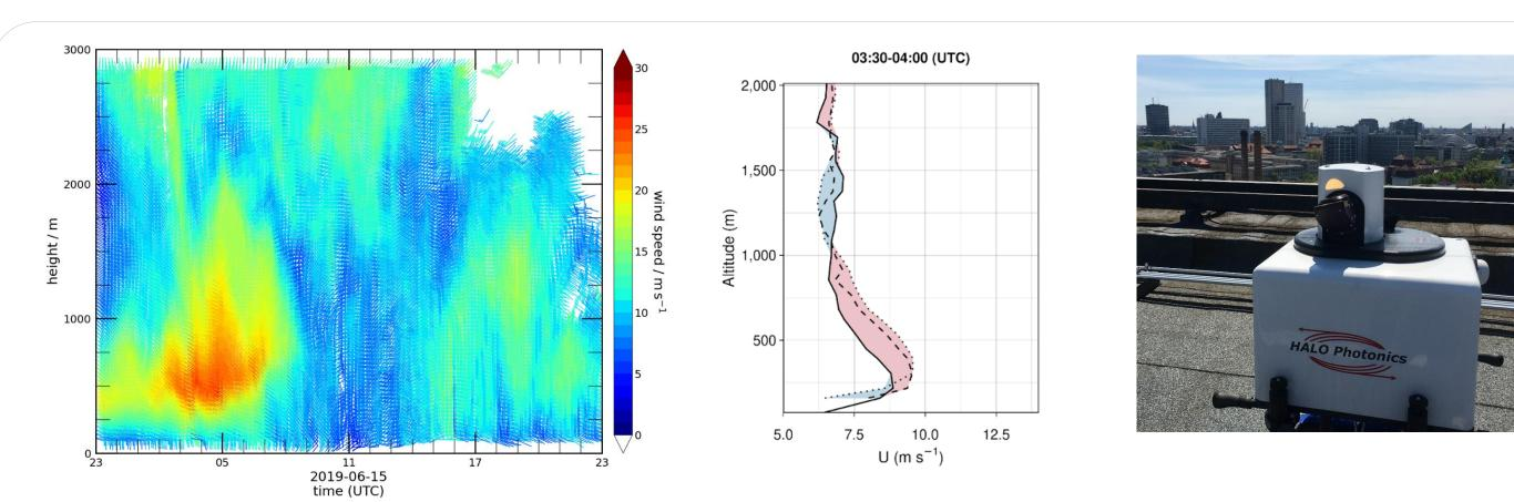
Ground-based remote sensing is used to study the urban boundary layer. UCO Berlin operates two Doppler LiDAR systems (Streamline XR, Halo Photonics) since 2018 and provides vertical profiles of wind speed and wind direction as well as information on atmospheric turbulence. The mid figure shows average vertical profiles of wind speed for the sites ROTH, TUCC and DWD-Lindenberg (solid line) and differences regarding nocturnal low-level jets.
