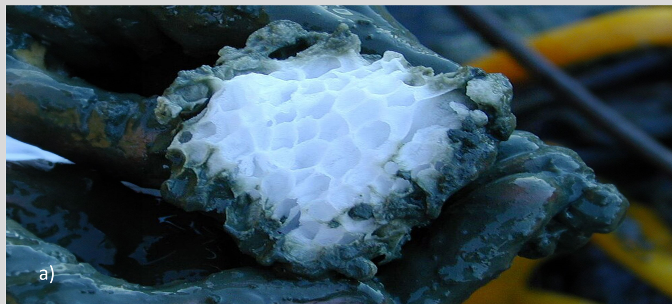
Fig.1. (a) Extracted gas hydrate sample. Retrieved from https://en.wikipedia.org/wiki/Clathrate_hydrate (b) Methane hydrate composition.
