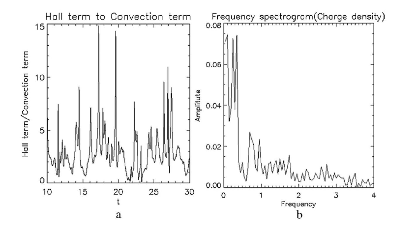
Fig. 1 Hall term compared to frozen-in term and frequency spectrogram of charged ion at the reconnection point in the case with guide field (Bg = 0.5) (a) The total value of the Hall term compared to the convection term. (b) The frequency spectrogram of ion charge density at the
