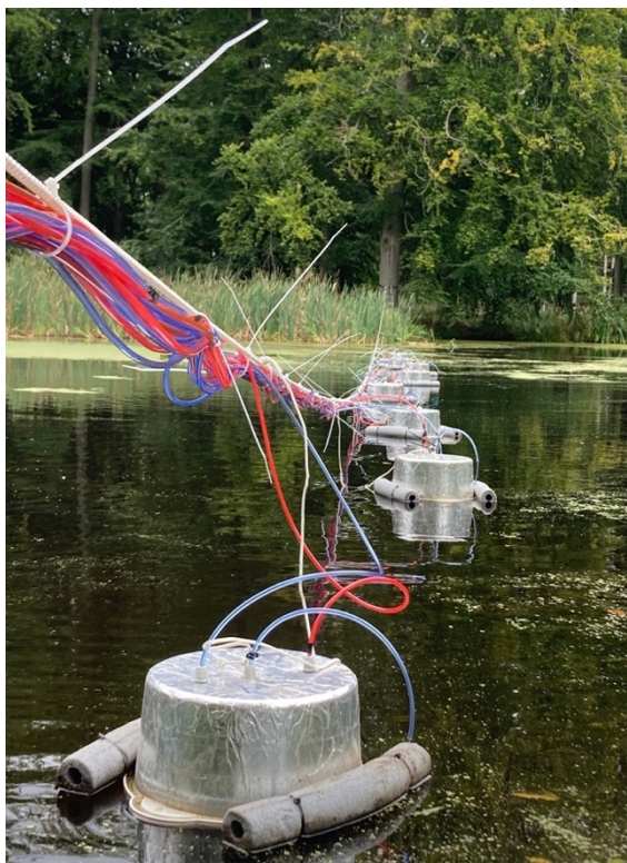
Picture 2: Picture from the field study. Eight AC attached to a rope tied between two trees across the pond.
