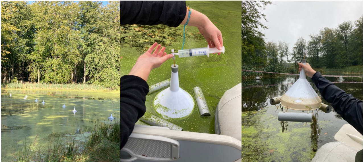
Picture 3: Pictures from the field study. Left: The eight BT located on a transect. Middle: Gas sampling from a BT. Right: BT during 'reset' after gas sampling.
