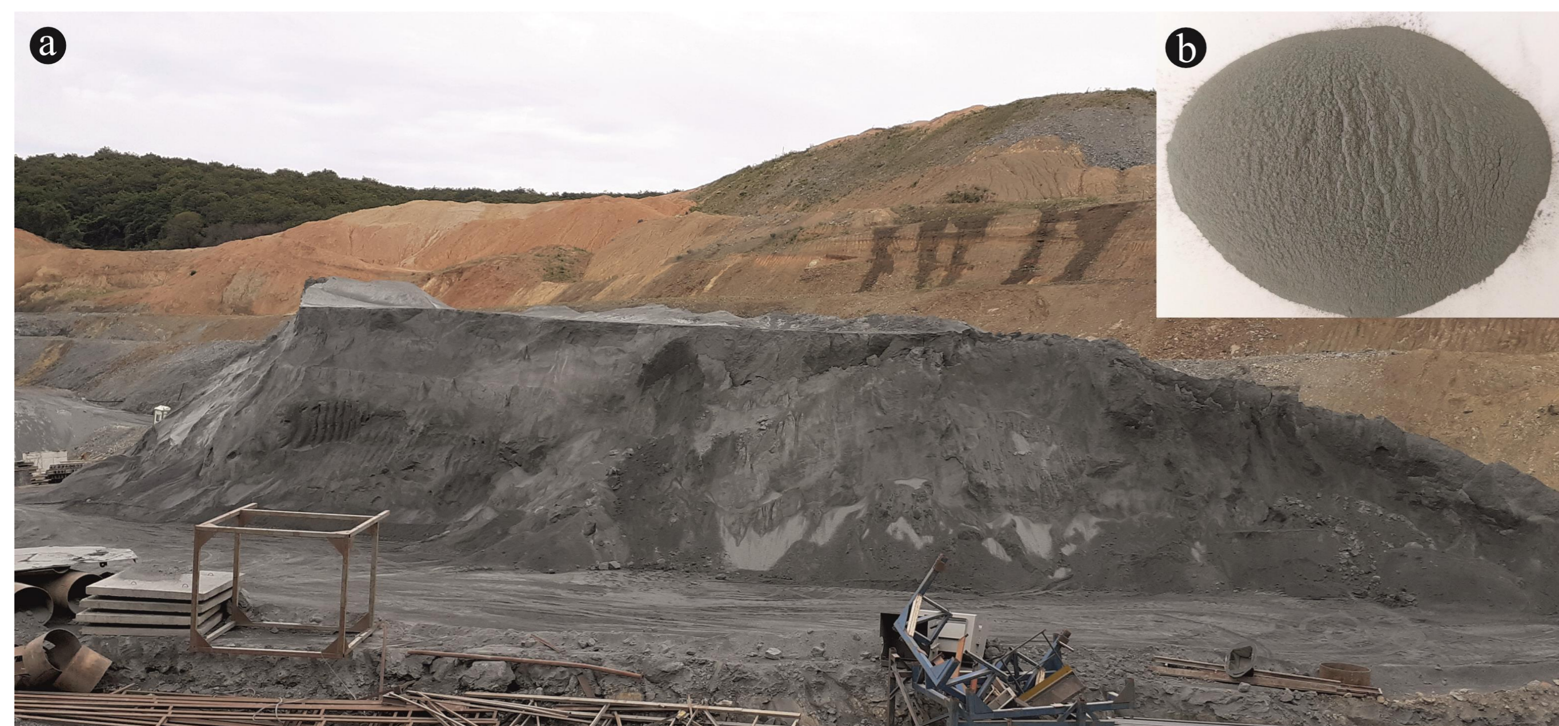
Figure 2: a-Fine aggregate containing clay with grain diameter less than 5 mm, b-100 µm sieved waste sample
