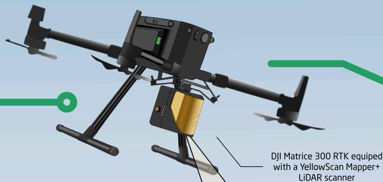
DJI Matrice 300 RTK equipped with a YellowScan Mapper+ LiDAR scanner
