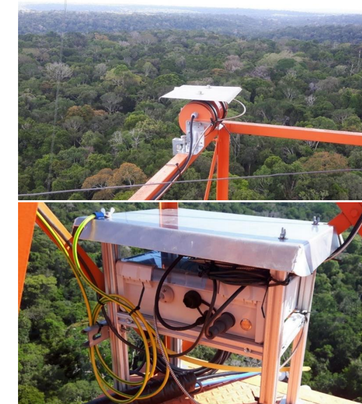
Fig. 3: MAX-DOAS instrument mounted on the ATTO tower.
