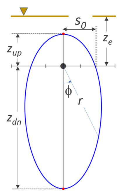
The above dimensional relationships also allow practical applications, as determining the water volumes required to achieve an assigned vertical bulb length. To
