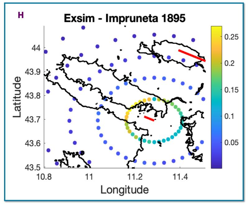
The Mugello and Impruneta's ground motion has been evaluated at epicentral distances ranging from 10 to 100 km Figure K using EXSIM to compute 360 synthetic waveforms in the high-frequency band (Figure G, H).
