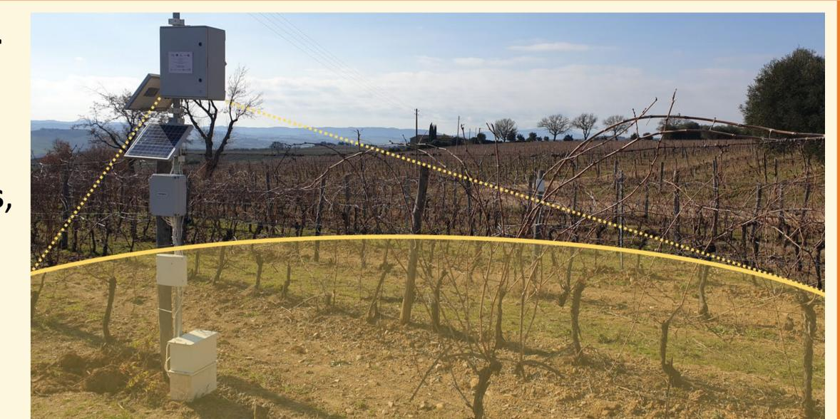
The **SWC value**  $\left[\frac{\text{kg}}{\text{kg}}\right]$  is determined from the **Counts Per Second (CPS)** using the formula:  $SWC\left(t\right) = \frac{A}{CPS\left(t\right)} + B$
