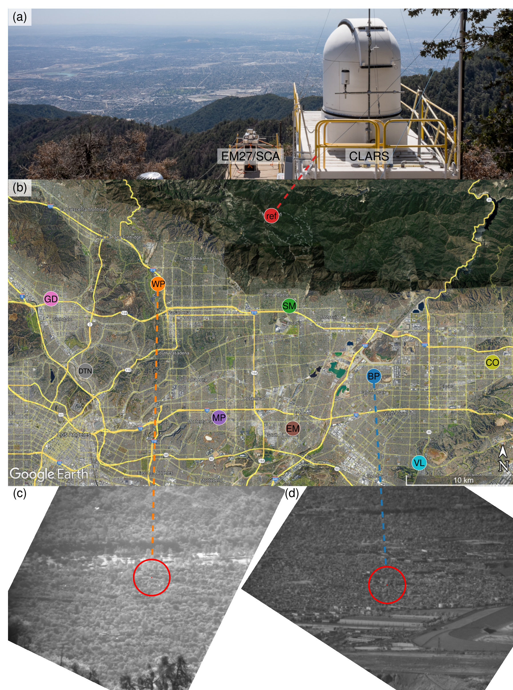
Figure 3: The EM27/SCA and the CLARS-FTS (Fu et al. 2014) side-by-side on Mt. Wilson (ref) observing nine ground scattering targets (other colored markers) in the LA Basin. The lower panels show FOV camera images of the West Pasadena (WP, c) and Baldwin Park (BP, d) targets. The instrument FOV is marked with a red circle.
