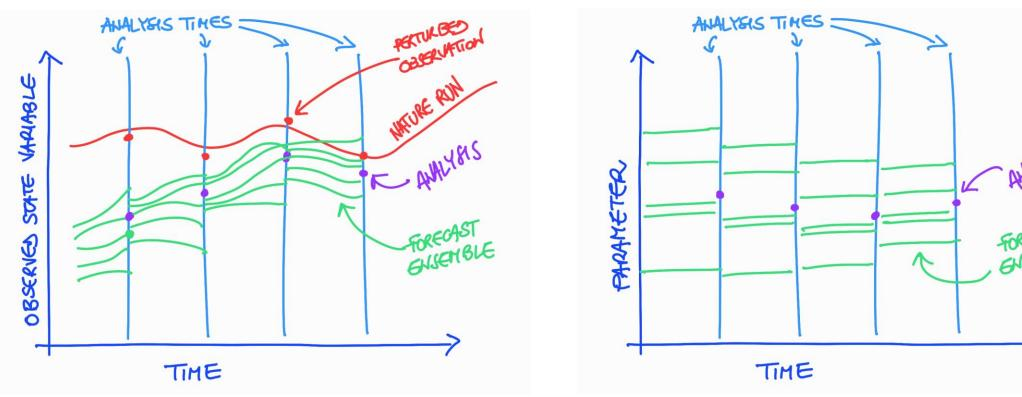
Parameter updates are determined by the ensemble correlations between parameters and model equivalents of the observations. For instance, using the Ensemble Adjustment Kalman Filter (EAKF):
