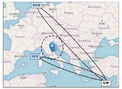
Location of the Norcia (Central Italy) earthquakes occurred at the end of October 2016. The dashed line encloses the Dobrovolsky area of the main shock (M w = 6.5, October 30, 2016); the ellipses define the 5 th Fresnel zones of the two radio paths
