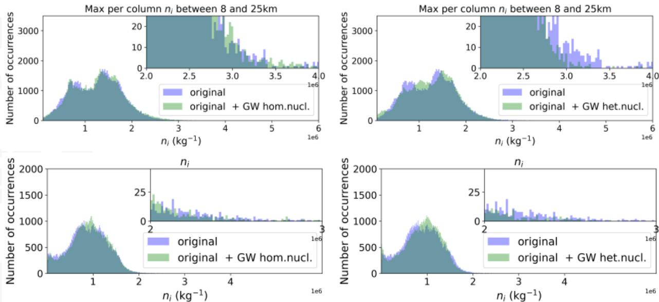
PDF of the maximum  $n_i$  per column (upper panel);  $n_i$  at 10km (lower panel).
