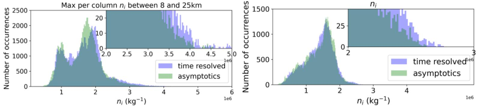
Figure: PDF of maximum per column  $n_i$  (left) and  $n_i$  at the 15km altitude (right)
