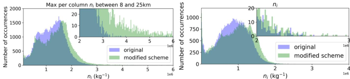
Figure: PDF of the maximum  $n_i$  per column (left),  $n_i$  distribution at 10km (right)
