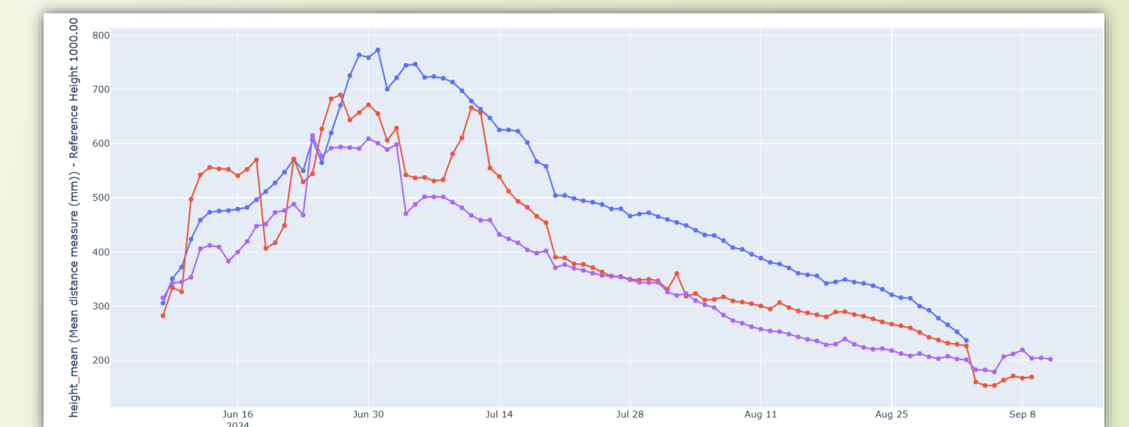
Mean Crop Height Calculated from the Lidar data of three CropTalker systems showing growth patterns in accordance with NDVI data
