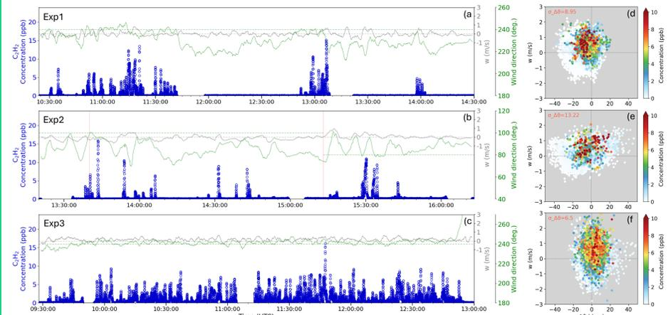
Figure 3. Time series (a-c) and quadrant analysis (d-f) of  $C_2H_2$  concentration, vertical wind speed ( $w$ ) and wind direction.  $\Delta\theta$  is defined as the difference between the wind direction and the azimuth angle from the tower to the releasing point.
