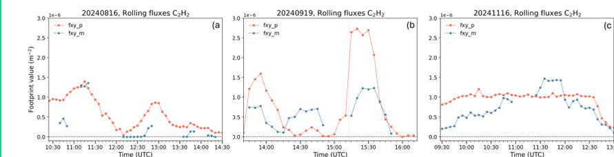
Figure 4. Comparison of the modelled footprint ( $f_{xy_p}$ ) and measured footprint ( $f_{xy_m}$ ) at release point.
