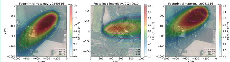
Figure 5. Footprint climatology of three TRE campaigns. White crosses (x) represent release points. The EC tower is located at (0, 0).
