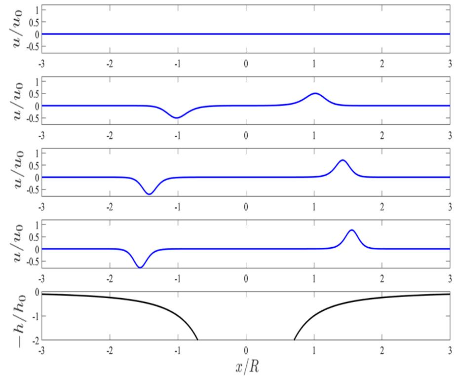
Evolution of the flow velocity along the non-reflective bottom geometry
