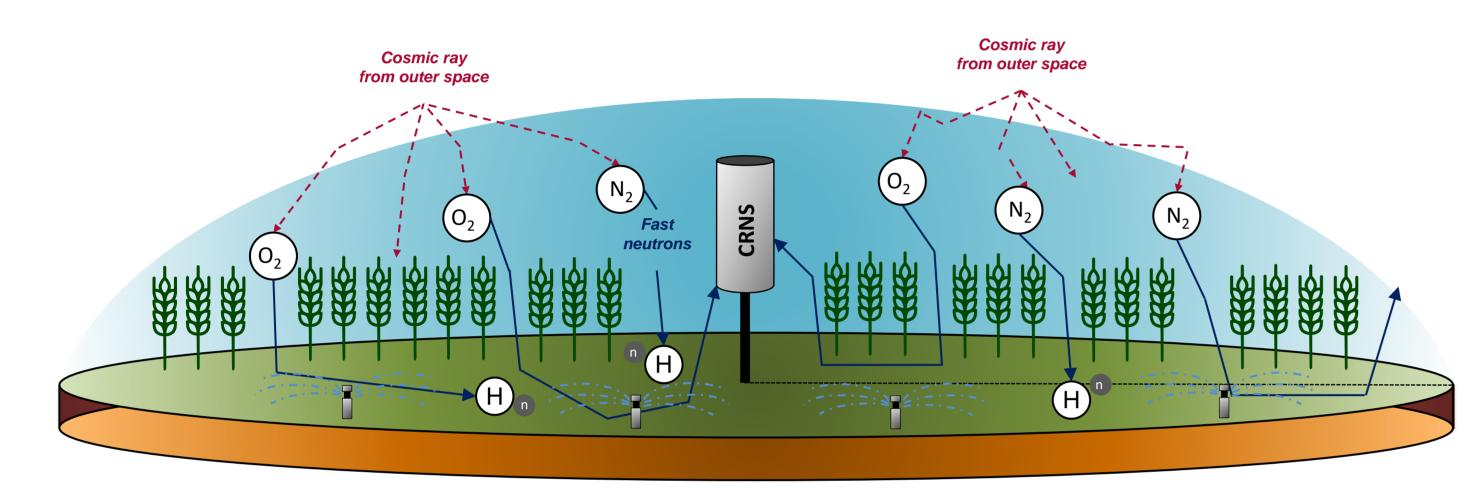
After multiple interactions with the environment, neutrons can reach the CRNS where depending on their energy, they can be detected
