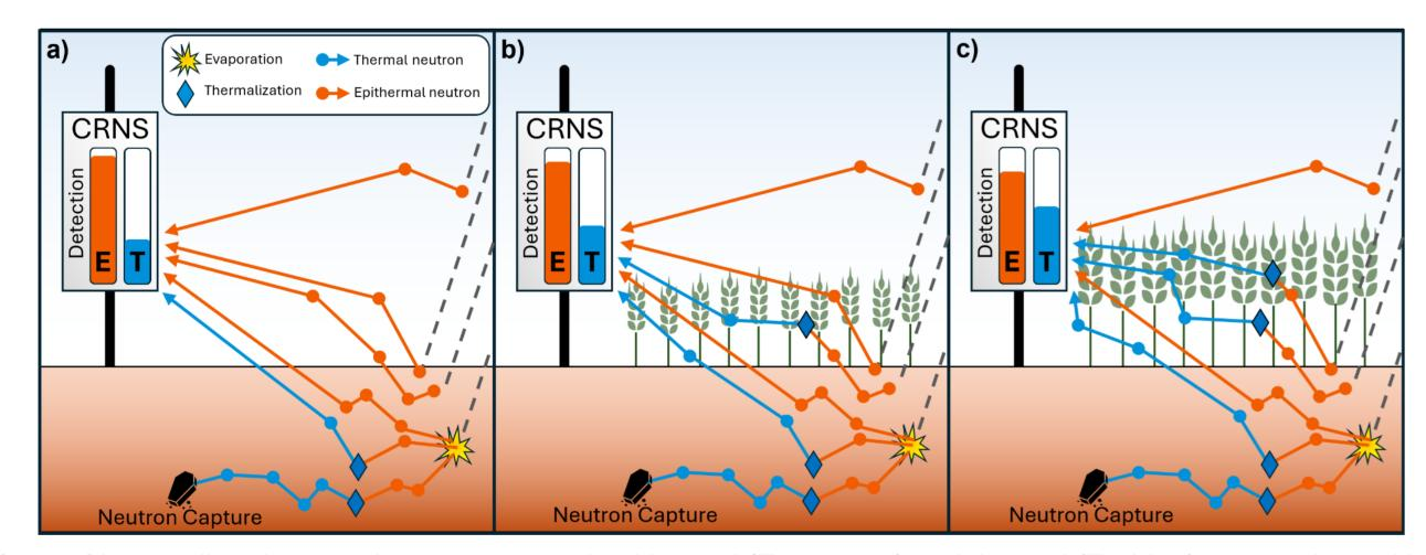
Effects of bare soil and vegetation on measured epithermal ( $E_n$ , orange) and thermal ( $T_n$ , blue) neutron intensities. Vegetation acts as an additional moderator and further slows down epithermal neutrons. With vegetation, En decreases slightly while  $T_n$  increases.
