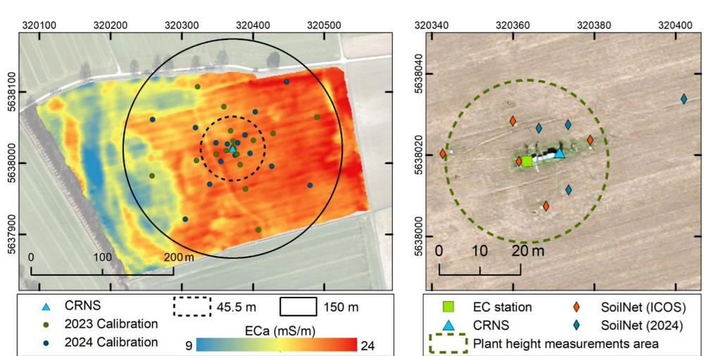
Study area with soil heterogeneity (apparent Electrical Conductivity, ECa), instruments and measurements positions, and CRNS footprints.
