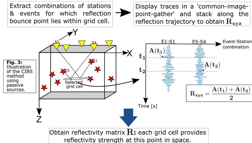
Fig. 3: Illustration of the CIBS method using passive sources.
