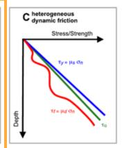
dynamic fault strength initial fault stress static fault strength
