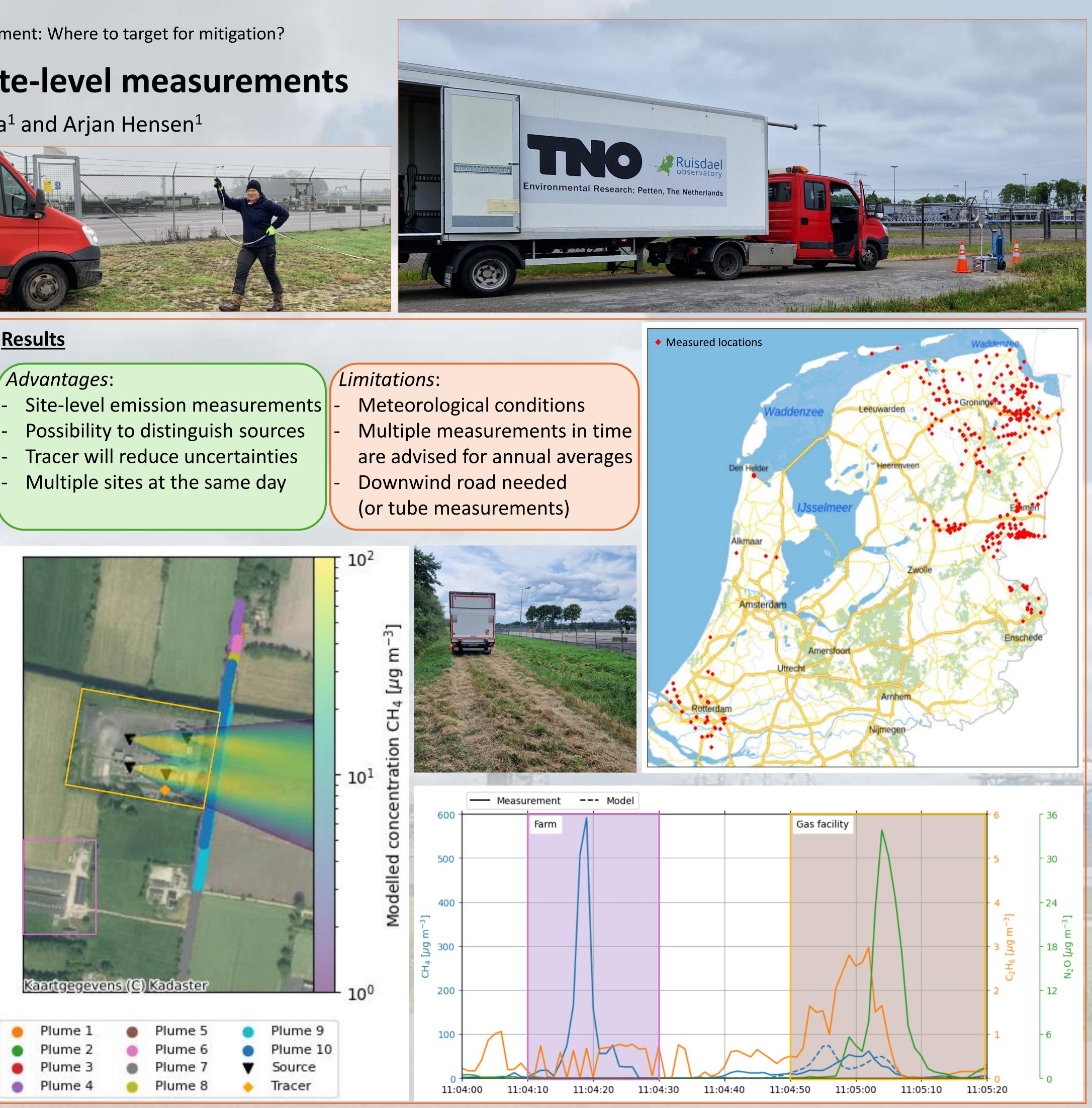
Conclusions This methodology not only complements source-level measurements but also improves the detection of previously unidentified emission sources, enhancing the overall reliability of emission inventories. Using a tracer will reduce the uncertainty significantly.
