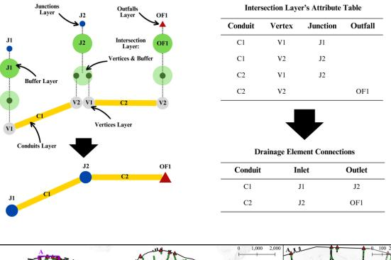
Batch processing in GIS allows instant connection of multiple drainage elements.
