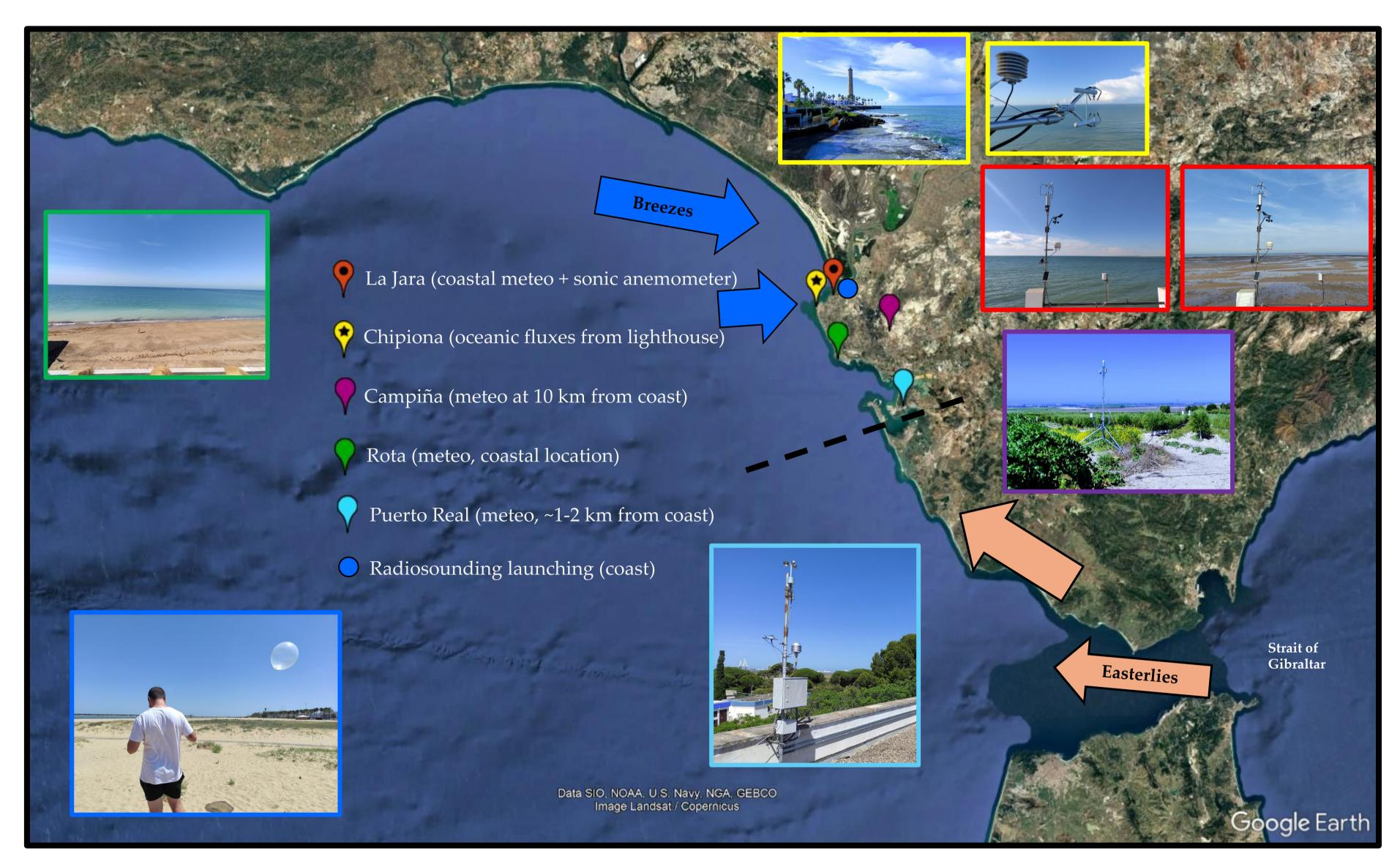
Coastal long-term stations strategically deployed to analyse the horizontal extension of the breezes, including both the location and pictures. Note how La Jara station includes a sonic anemometer at 10 m above sea level (asl) and the Chipiona station an IRGASON to measure energy fluxes from a lighthouse (68 m above sea level). All the stations were installed to avoid perturbations from winds coming from the sea. Radiosoundings were launched from coastal locations during sea breeze events.
