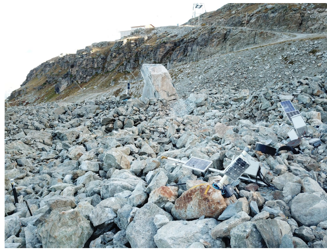
Fig.3 Field photograph of destroyed measurement station at Murtèl-Corvatsch
