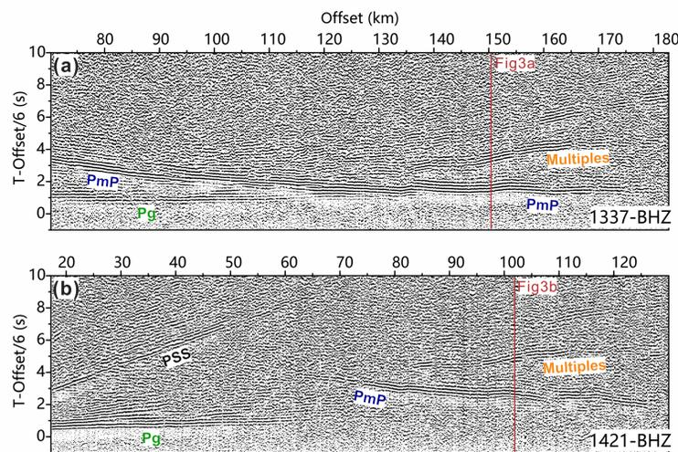
Fig.2 The air gun signal recorded by the land stations show seismic multiples. The crustal refraction phase (Pg), Moho reflection phase (PmP), and multiples can be clearly identified.
