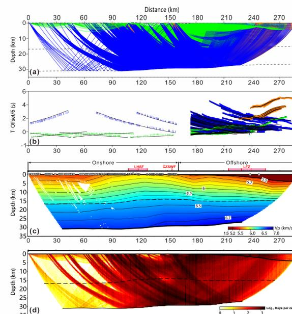
Fig.6 P-wave velocity model along the L1-NW03 survey line. P-wave velocity model with contour intervals of 0.1 km/s.
