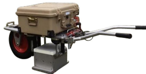
The vibrator source with the horizontal vibrator kit (mounted).
