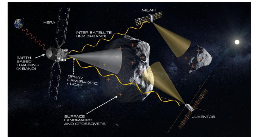
**Figure 1:** Hera radio science experiment measurement model. The measurements included within the Hera RSE are ground-based radiometric data, Hera optical images, Hera to CubeSats Inter-Satellite Link radiometric measurements, and Hera PALT LIDAR measurements to surface landmarks and crossovers on Didymos and Dimorphos.
