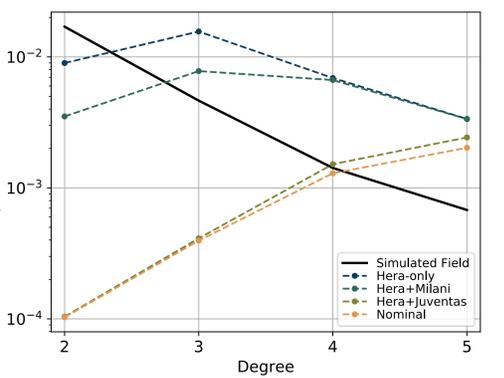
**Figure 5:** Power spectra of the simulated Didymos gravity field (black) and of the recovered gravity field uncertainty at the end of the nominal mission, showing the contribution of each spacecraft.
