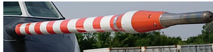
Meteorology (p, T, u, v, w) up to 100 Hz
