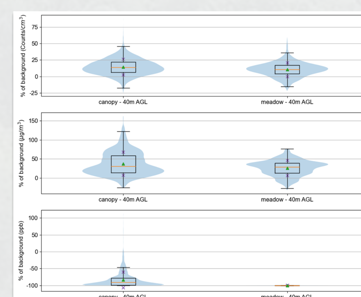
Fig 3. Comparison of total particle concentration (POPS), PM 2.5 (SEN55), TVOC (CCS811) to a pre-flight period over all flights
