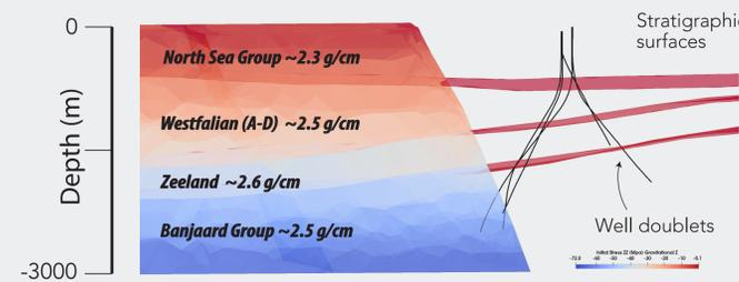
Initial stress zz condition is computed from integrating gravitational force from formation densities
