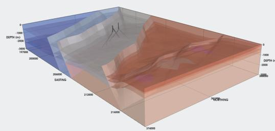
3D meshed volume from structural model realizations
