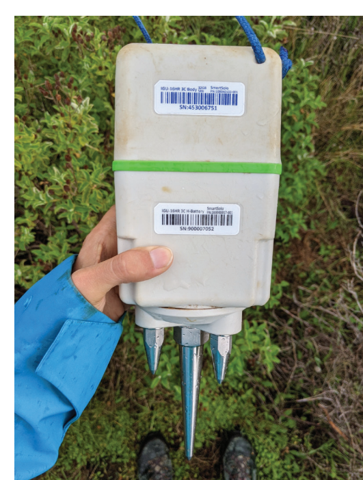
Figure 2: Nodal geophones are discreet and require minimal planning and permitting to deploy. Here a geophone used in Thurgau, manufactured by SmartSolo (IGU16HR-3C 5Hz)
