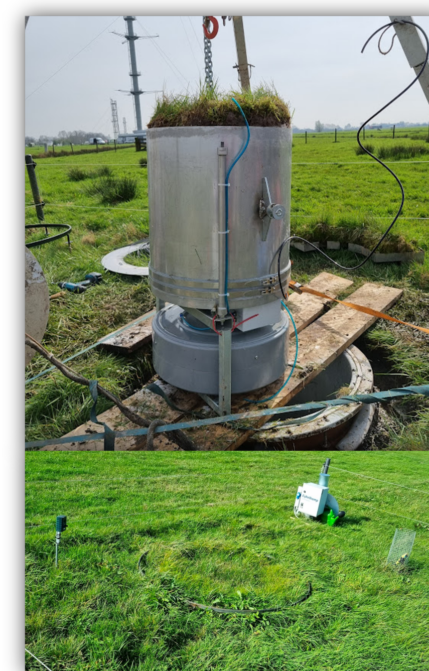
Figure 4: Smart lysimeter before (upper panel) and after (lower panel) being deployed. Also pictured below is the tensiometer which measures the surrounding field soil water tension.
