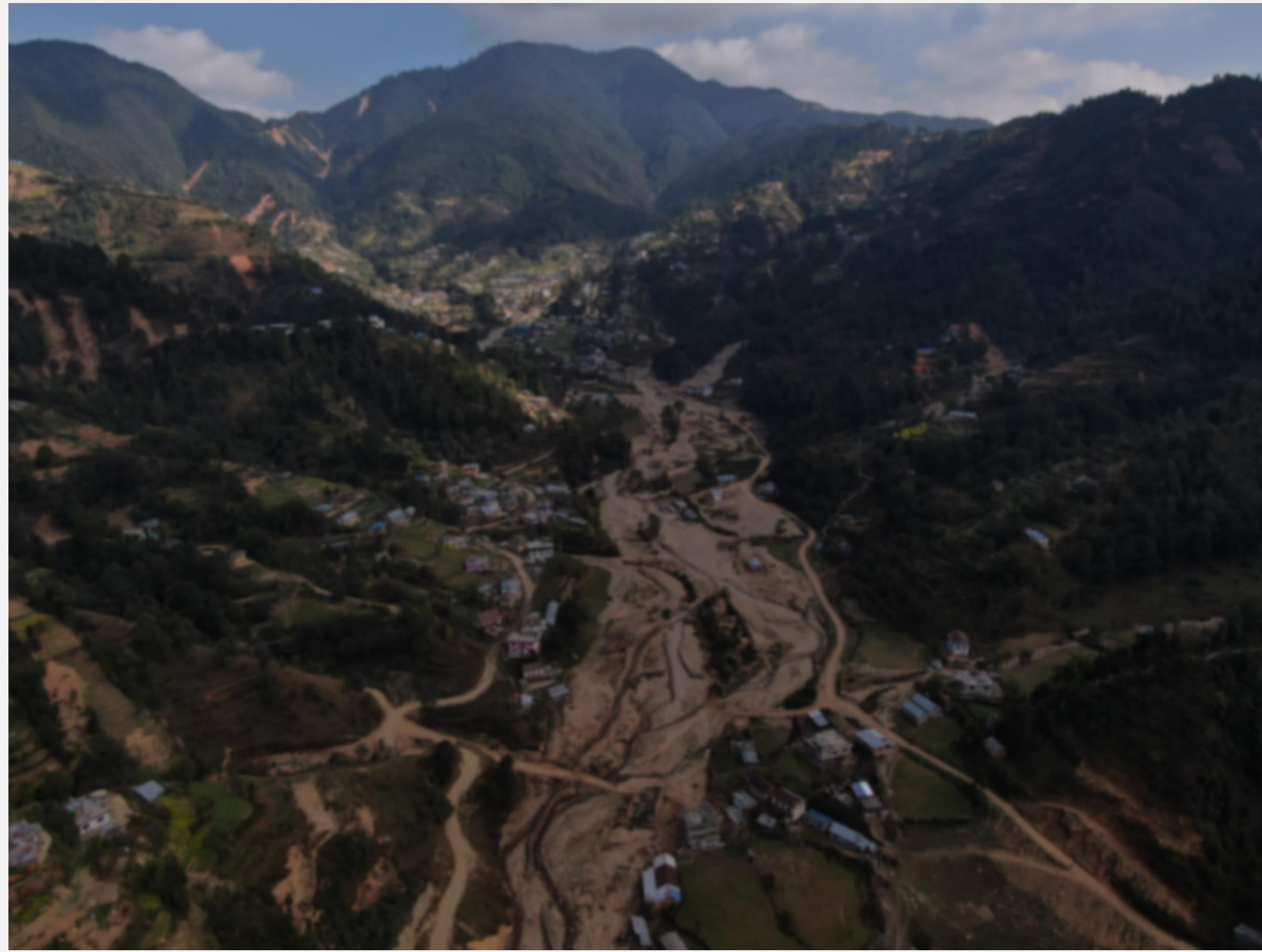
Fig. 3 Rainfall triggered compound sediment disasters, raising the river ~3 m above the riverbed, along with landslides and debris flows. Shallow landslides primarily occur along roads and cultivated land areas.
