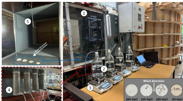
**Fig. 1:** Wind tunnel experimental setup: (1) Optical camera, (2) Mariotte bottles, (3) Balances, (4) Sample columns, and (5) Prandtl tube. The inset shows the surfaces of the samples exposed to a wind velocity of 5 m/s
