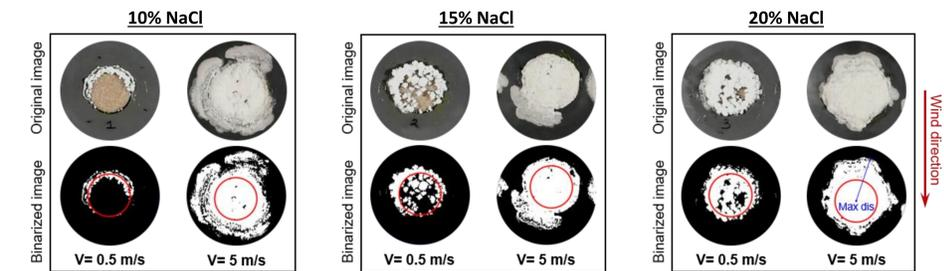
**Fig. 5:** Salt precipitation patterns of sample saturated with 10%, 15%, and 20% NaCl solutions under 0.5 m/s and 5 m/s wind velocities.
