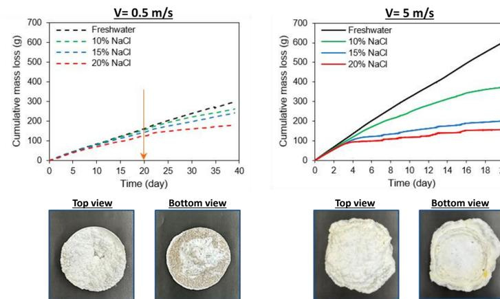
**Fig. 3:** (top) Cumulative mass loss versus time for samples saturated with 0%, 10%, 15%, and 20% NaCl concentrations under wind velocities of 0.5 m/s and 5 m/s. (bottom) The top and bottom views of salt crystals from samples saturated with 20% NaCl at the end of experiments at two wind velocities.
