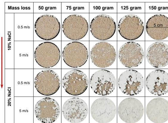
**Fig. 4:** Surface images of samples saturated with different NaCl solutions under wind velocities of 0.5 and 5 m/s, presented with their respective water mass loss.
