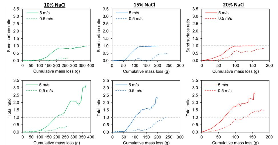
**Fig. 6:** Evolution of salt crystal (projected) area as a function of cumulative mass loss for samples saturated with different NaCl concentrations, exposed to wind velocities of 0.5 m/s (dashed lines) and 5 m/s (solid lines): (top) coverage ratio over the sample surface; (bottom) coverage ratio over the combined sample surface and supporting plate (total). The coverage ratios are estimated based on the column surface area with a diameter of 5 cm.
