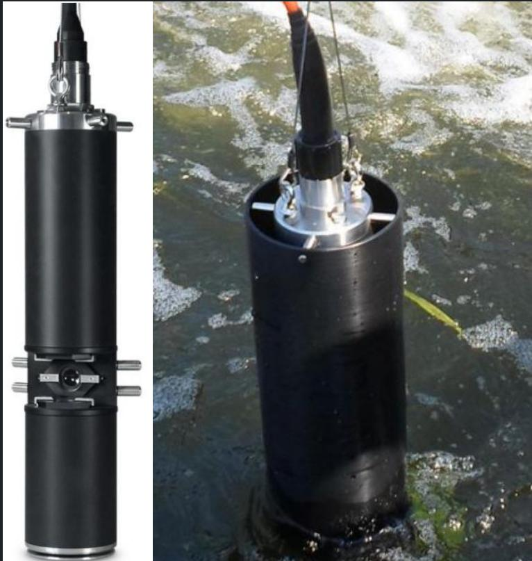
Figure 21. Biological biophysical engineering (bbe) moldaenke FluoroProbe (bbe moldaenke GmbH 2025).
