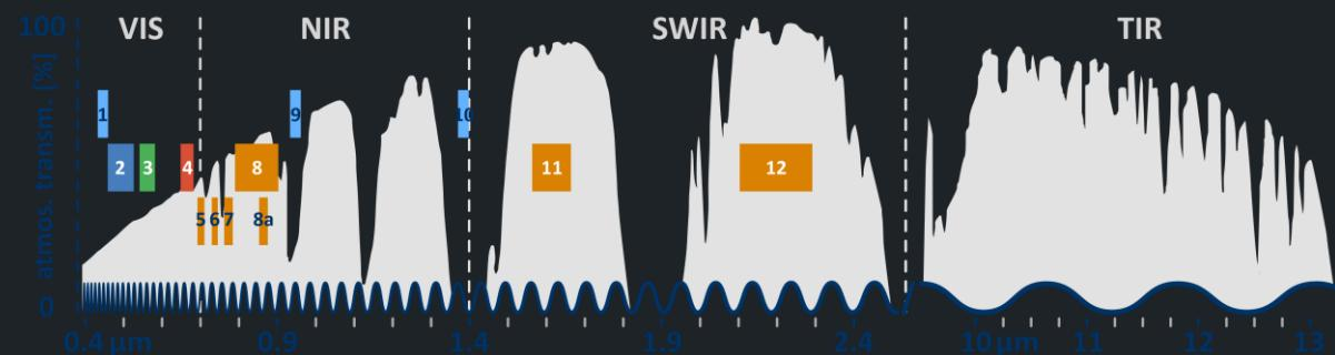
Figure 3. Sentinel-2 MSI bands on the electromagnetic spectrum (FU Berlin 2024).
