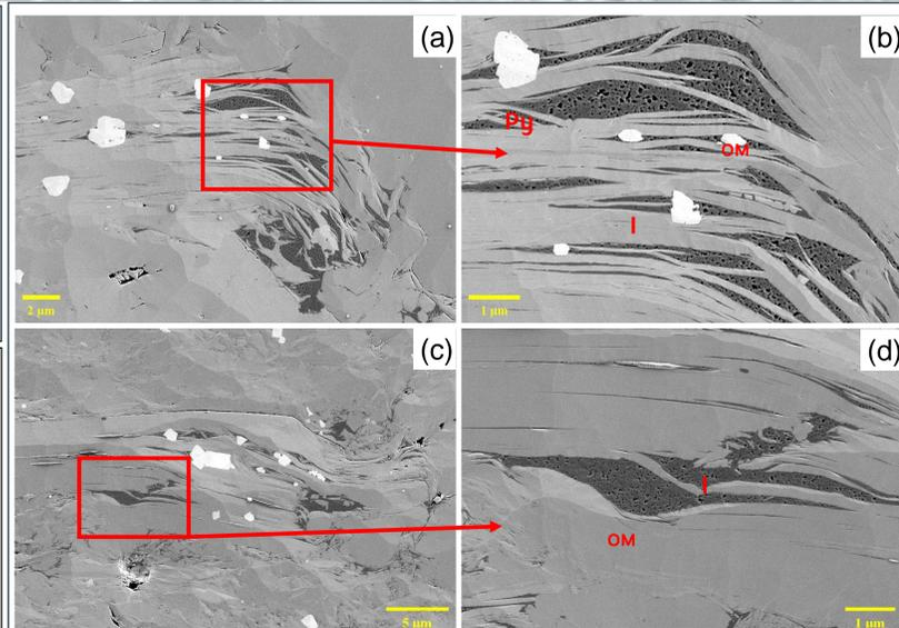
Figure 3. Syngenetic clays preserving OM-hosted pores: TY1, (a) and (b); N206, (c) and (d).
