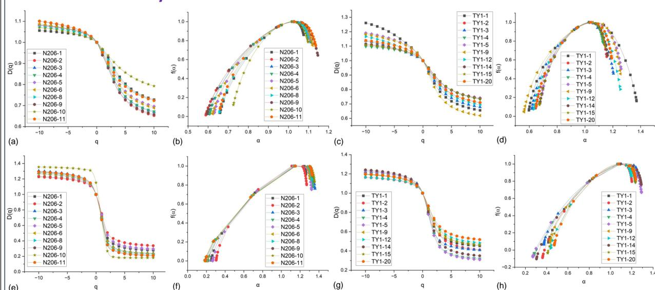
Figure 7. Relationship between D<sub>q</sub> and q from low pressure CO<sub>2</sub> adsorption isotherms for (a) N206 and (c) TY1; Multifractal singularity from low pressure CO<sub>2</sub> adsorption isotherms for (b) N206 and (d) TY1; Relationship between D<sub>q</sub> and q from low pressure N<sub>2</sub> adsorption isotherms for (e) N206 and (g) TY1; Multifractal singularity from low pressure N<sub>2</sub> adsorption isotherms for (f) N206 and (h) TY1.
