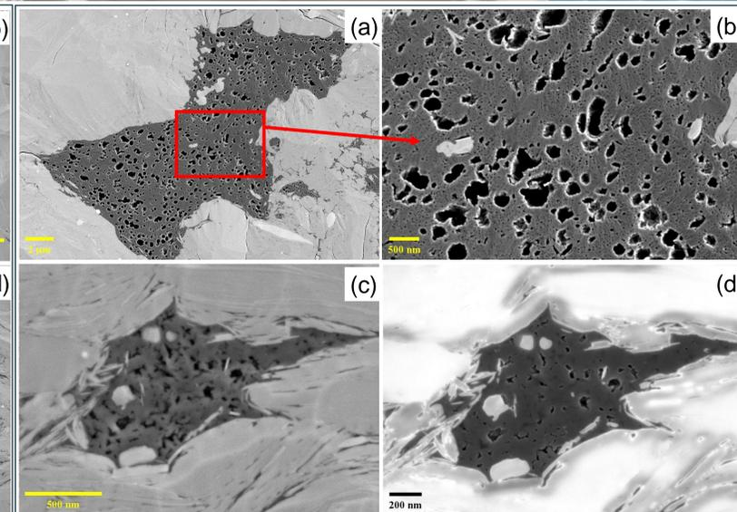
Figure 5. OM-hosted pores comparison: TY1, (a) and (b); N206, (c) and (d).
