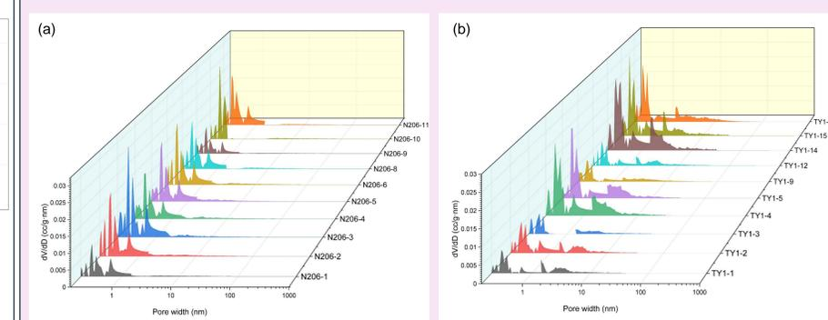
Figure 8. Pore size distributions obtained from MIP and low-pressure gas (CO<sub>2</sub> and N<sub>2</sub>) sorption analysis: (a) N206; (b) TY1
