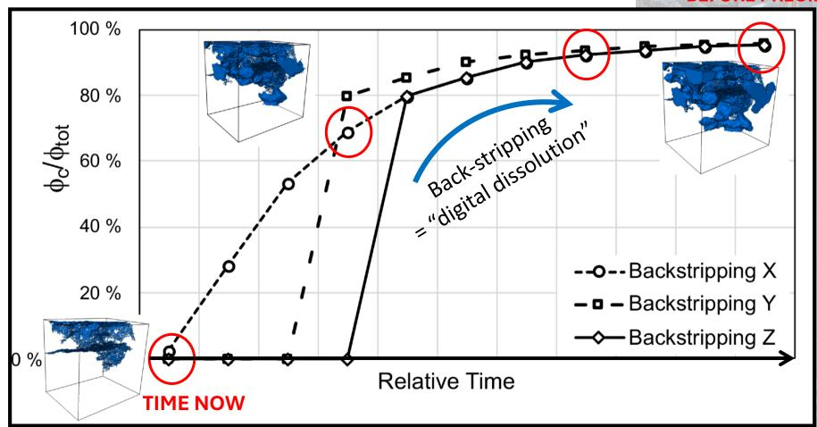
Porosity is more connected along the X direction, along which the fracture network develops.
