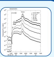
Intensity-time profiles at different energies for an event detected on the 19th October 1989 by one of the Geostationary Satellites launched by NOAA
