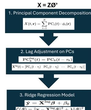
Fig.2a: PCA+ Ridge Regression Architecture.
