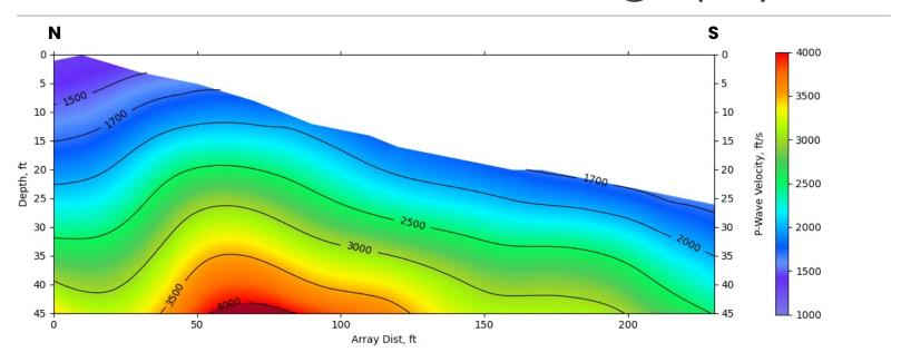
Vp triggerless tomographic results Geocon collected during field training with Terean showing bedrock at 40 ft depth.
