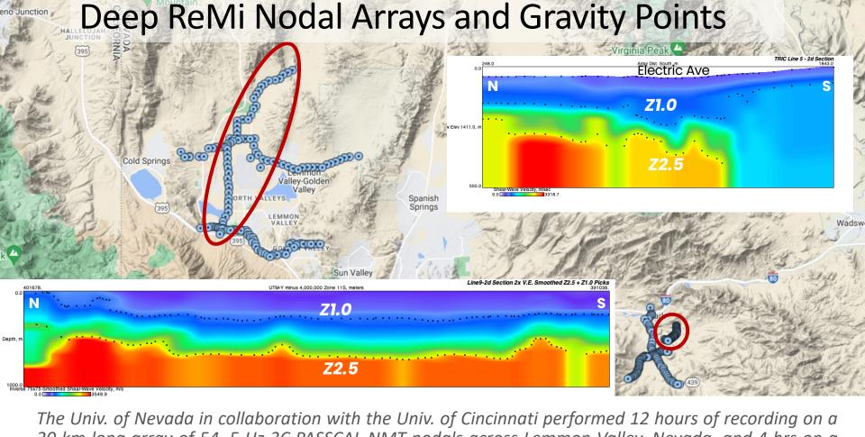
The Univ. of Nevada in collaboration with the Univ. of Cincinnati performed 12 hours of recording on a 20 km-long array of 54, 5 Hz 3C PASSCAL-NMT nodals across Lemmon Valley, Nevada, and 4 hrs on a 2 km array across Electric Ave. in TRIC. Deep ReMi shear-wave velocity sections from Terēan analyses.
