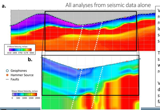
Vp triggerless tomographic results (a) are correlated with Vs results (b). Inferred fault locations projected. Seismic sections are plotted relative to surveyed geophone locations.
