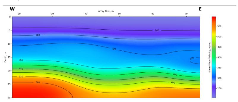
Suelo-Estructura in Guadalajara, Jalisco, Mexico used ReMi 2dS™ software to <u>determine the depth and</u> <u>thickness of layers and bedrock topography</u>. Variations in subsurface bedrock topography are required for rippability, determining overburden removal costs, and placement of engineered structures.
