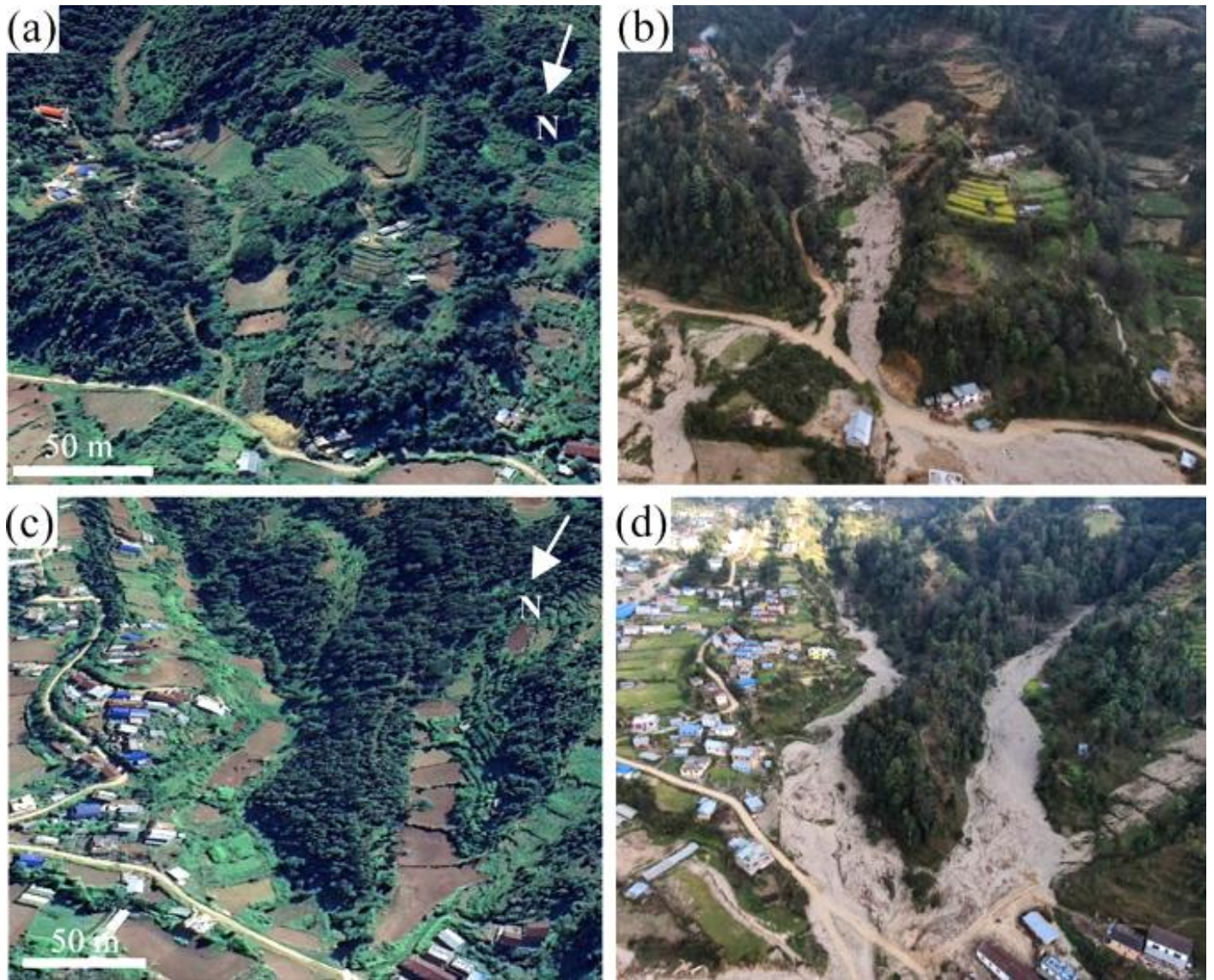
Supplementary Fig.6. Condition of unmitigated creek (a) Gully ca. 300 m upstream of Creek No. 8 before the rainfall event (Google Earth image, September 23, 2023). (b) Same gully of Fig. 15a after the rainfall event (photo taken on November 24, 2024). (c) Gully ca. 600 m upstream of Creek No. 8 before the event (Google Earth image, September 23, 2023). (d) Same gully of Fig. 15c after the event (photo taken on November 24, 2024).
