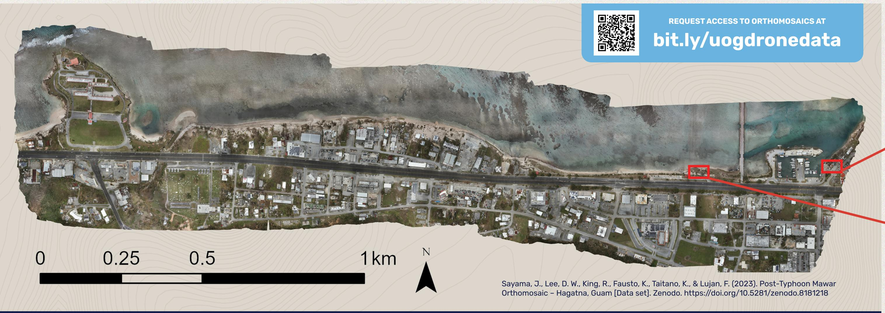
An orthomosaic map of Hagåtña, Guam following the passage of Typhoon Mawar. This orthomosaic was created from 1974 images taken on 27 May 2023, at 121.92m AGL, with a DJI P1 Sensor mounted to a DJI Matrice 300 UAV.
