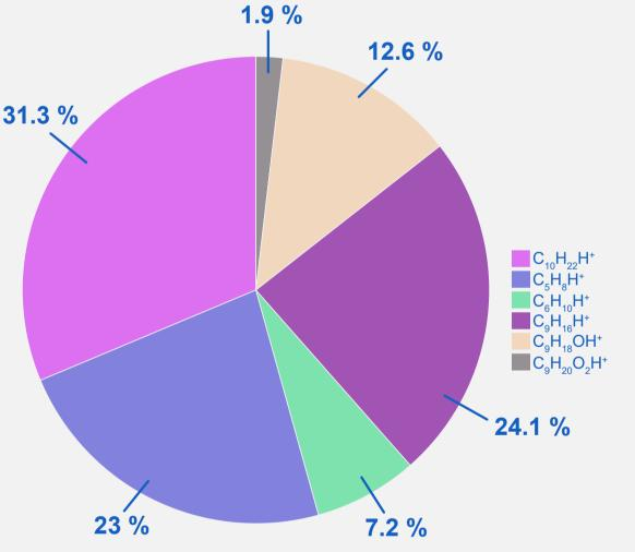
$C_5 H_8 H^+$  peak likely arising from fragmentation of higher molecular weight aldehydes. Specific ion attribution requires separation prior to analysis on the PTR-ToF-MS
