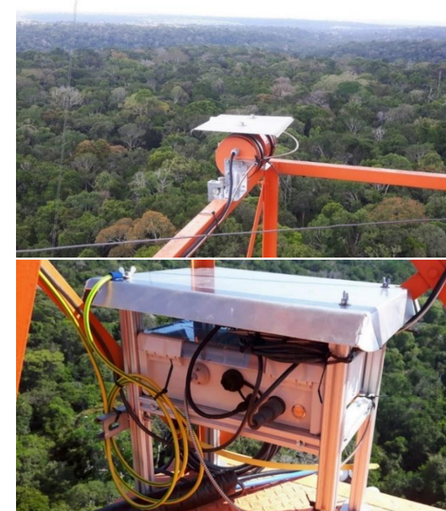
Fig. 3: MAX-DOAS instrument mounted on the ATTO tower.
