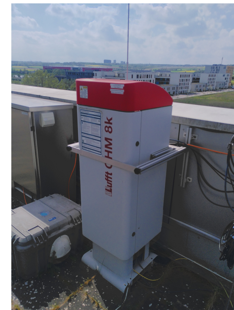
Figure 3: Rooftop Ceilometer, located next to the Cloud Camera and MAX-DOAS instrument.
