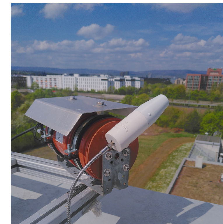
Figure 4: Photograph of the MAX-DOAS instrument scanning at 30^\circ elevation angle.
