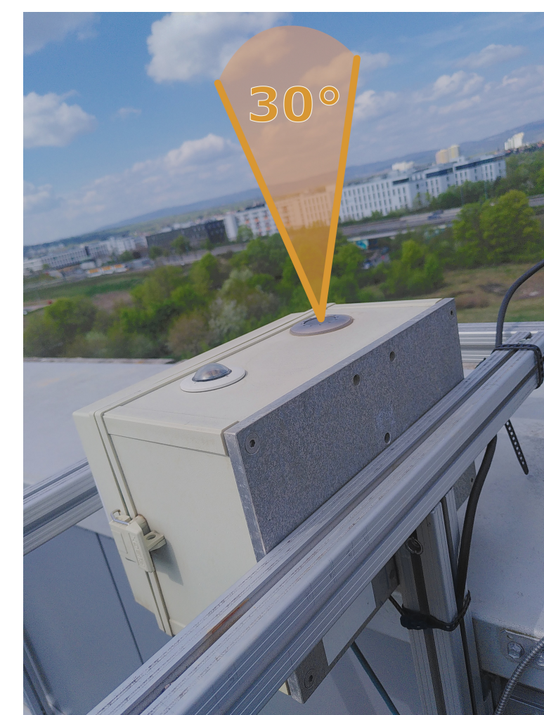
Figure 1: Cloud Camera with the IR viewing angle of 30° drawn in.
